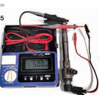
The meter allows to diagnose coil and piezoelectric injectors for short circuits It enables measurement at 250V (and higher) voltage and 1mA test current.
