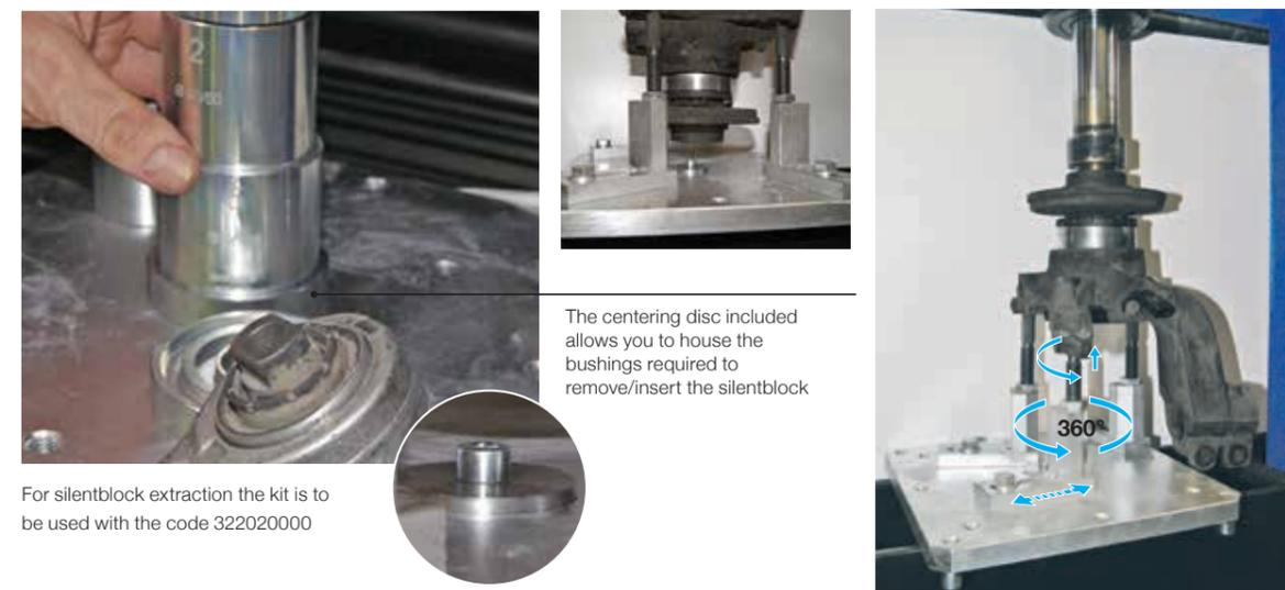
For silentblock extraction the kit is to be used with the code 322020000
