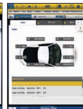
Possibility of connect to a TPMS control unit for its configuration or to assign new sensor codes.
