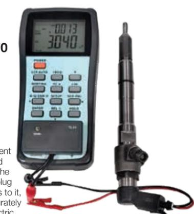
Device allows for accurate measurement of the resistance and continuity between the pins of the injector plug and its body. Thanks to it, it is possible to accurately assess the piezoelectric stack capacity in piezoelectric injectors.
