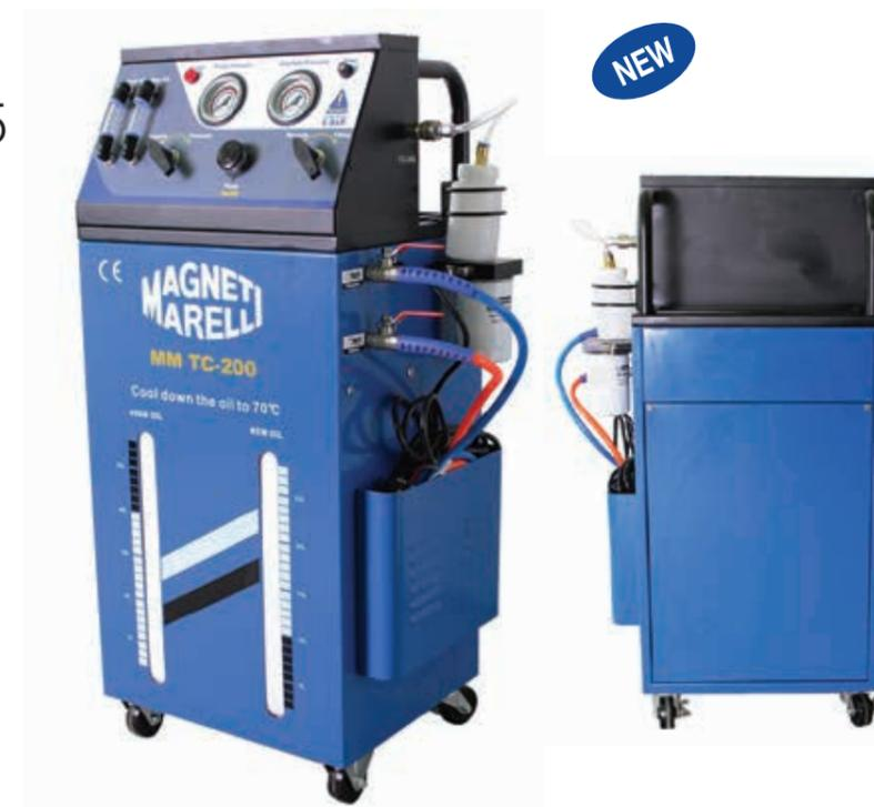
The **MM-TC200** device allows you to drain the gearbox from used oil, flush it with a appropriate detergent, and fill it with fresh oil up to the level recommended by the manufacturer. Unlike the previous version of the device, the MM-TC200 uses variable displacement pump, Parker quick couplers, new hoses inside the unit, and refreshed front panel.
