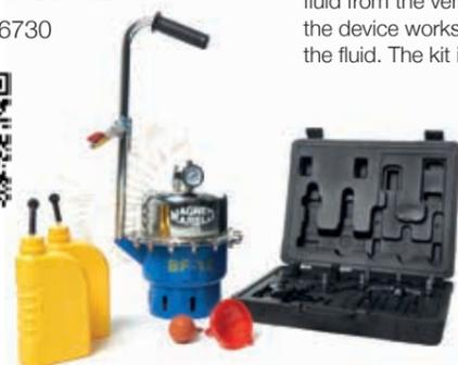
Universal pneumatic device for brake fluid replacement. The device consists of a stainless steel container, inside which a rubber diaphragm moves, sucking the brake fluid from the vehicle. After filling the internal tank to maximum operating pressure, the device works independently. Just one technician is required to completely replace the fluid. The kit includes service adapters, hoses and two 1-litre reservoirs.
